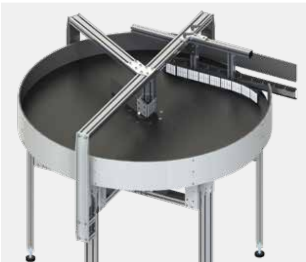
Separation during ejection via various guides
